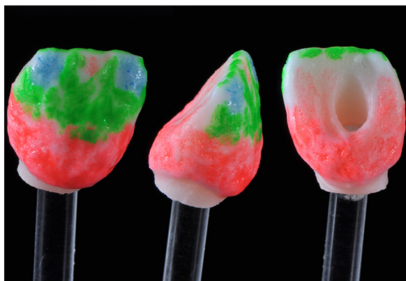
Fig. 7. The zirconia element covered with very thin layer of ceramic before firing.
